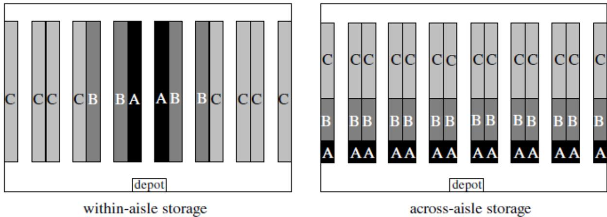
Figure 7 - Class based storage types (De Koster et al., 2007)
