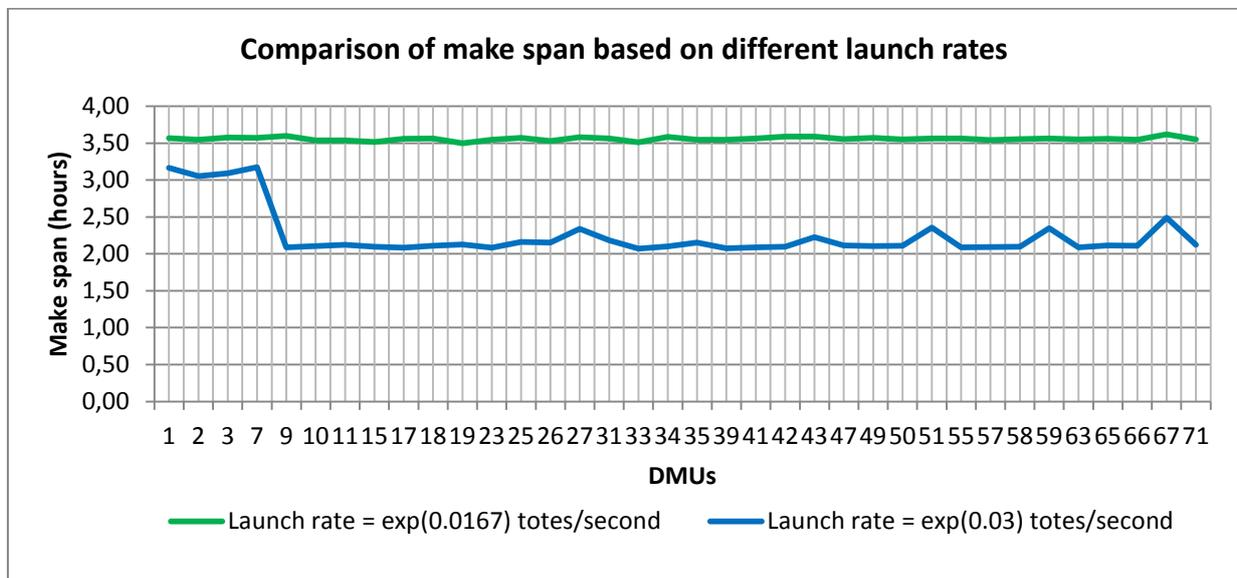
Figure 17 - Comparison of make span based on different launch rates
