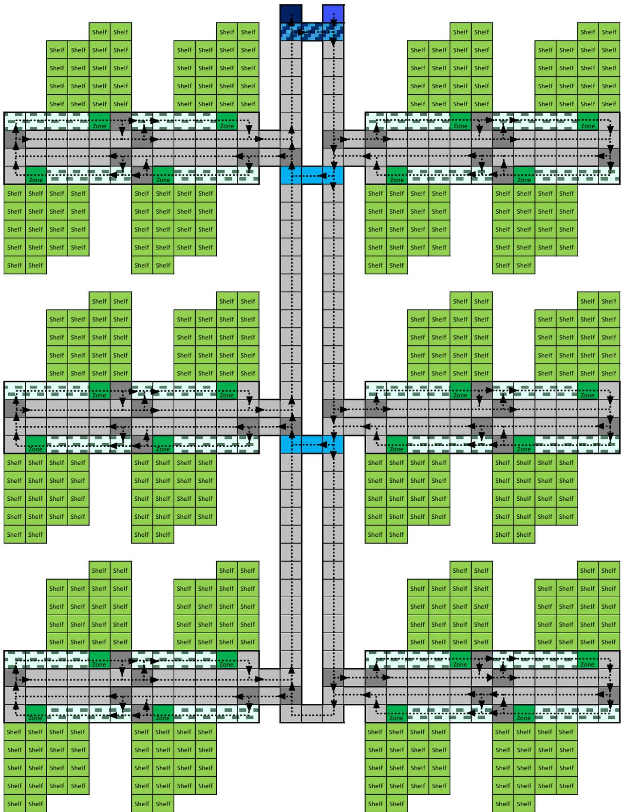
Figure 9 - Configuration of a model with 6 segments and 4 zones/ segment
