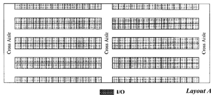
Figure 5 - Parallel aisles (Caron et al., 2000)
