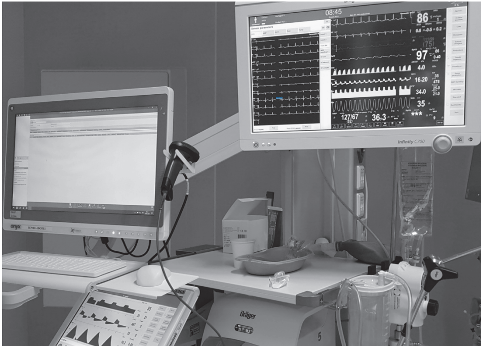
Figure 2: Some of the technologies inside an ICU patient's room: a vital sign monitor, a ventilator, and a computer displaying the patient's EHR.
