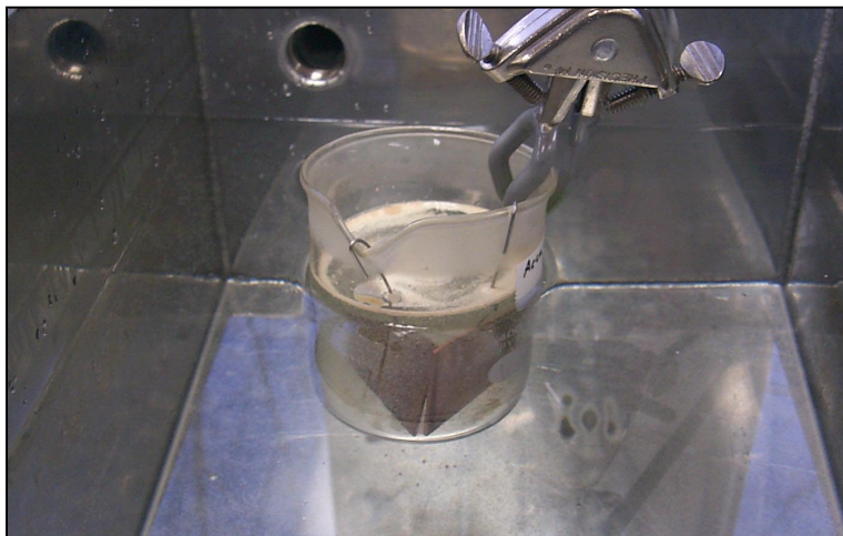
Figure 5.9 LAB ULTRASONIC TANK FILLED WITH WATER AND SUSPENDED TEST BEAKER
